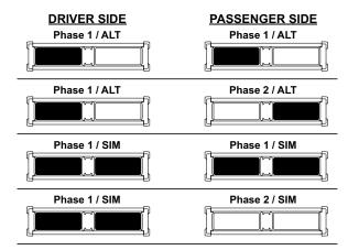
Synchronized lightbars, must be set to the same pattern. Not all patterns can be synchronized. Below are patterns available for SYNC.
