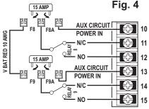
**Moving Fuse #8** from its default position (F8) to its optional position (F8A) allows push-
