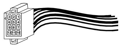
BLACK LEAD: (*Terminal 2*) – *Ground*: Connect to the negative of the battery, or to a good chassis ground. Be sure to use minimum size #14 AWG wire.
