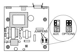
The unit is factory shipped with the horn option (AUX) defaulted to activation by applying a positive voltage to the wire (your vehicle horn switches +12VDC). To activate the Air Horn by connecting to ground or negative (your horn is Ground-side switched), move the "AUX" option jumper from the "POS" pins to the "NEG" pins. (See diagram above).
