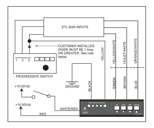
**IMPORTANT!:** Customer installed diode (i.e. 1N4004) shown above <u>MUST</u> be installed or damage to the Directional Arrow Switch could occur.
