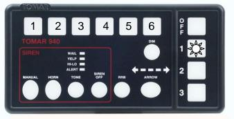
(a) Selecting Flash Pattern: Select the Mode 1 warning pattern by pressing the appropriate switch as listed below. Each press advances the pattern one step. Continue until the desired pattern is selected.
