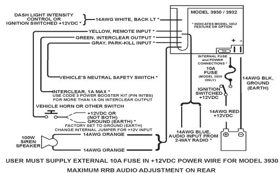
Figure 2 - Wiring Diagram
